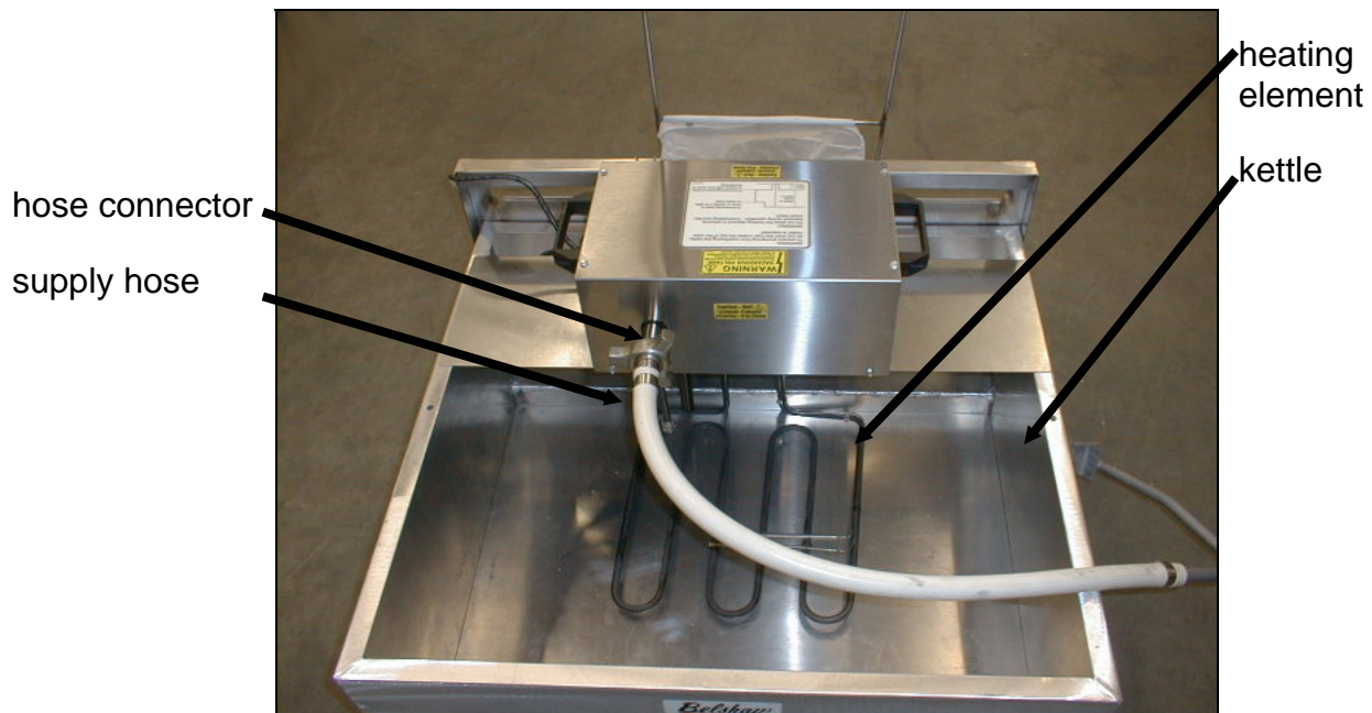
Figure 1-3. Top View, Heater Head.
